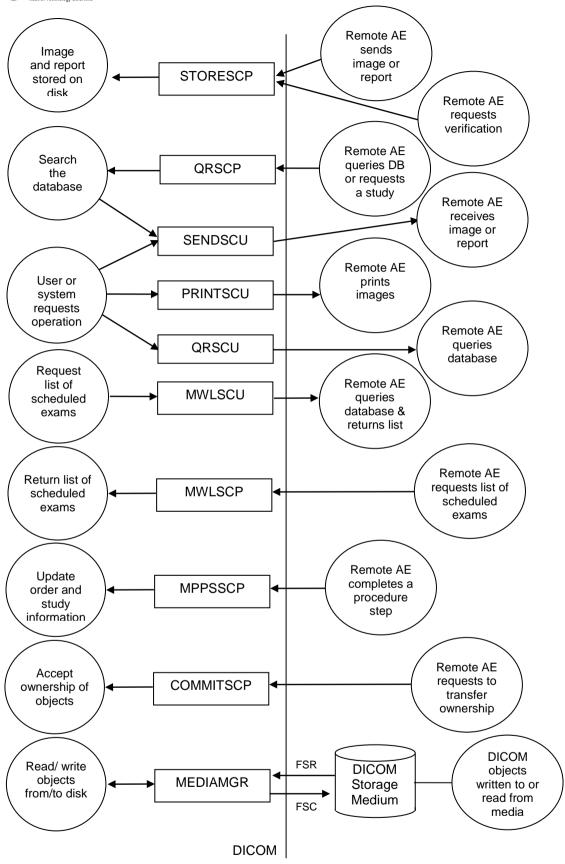
Figure 1.1-1 Application Data Flow Diagram
