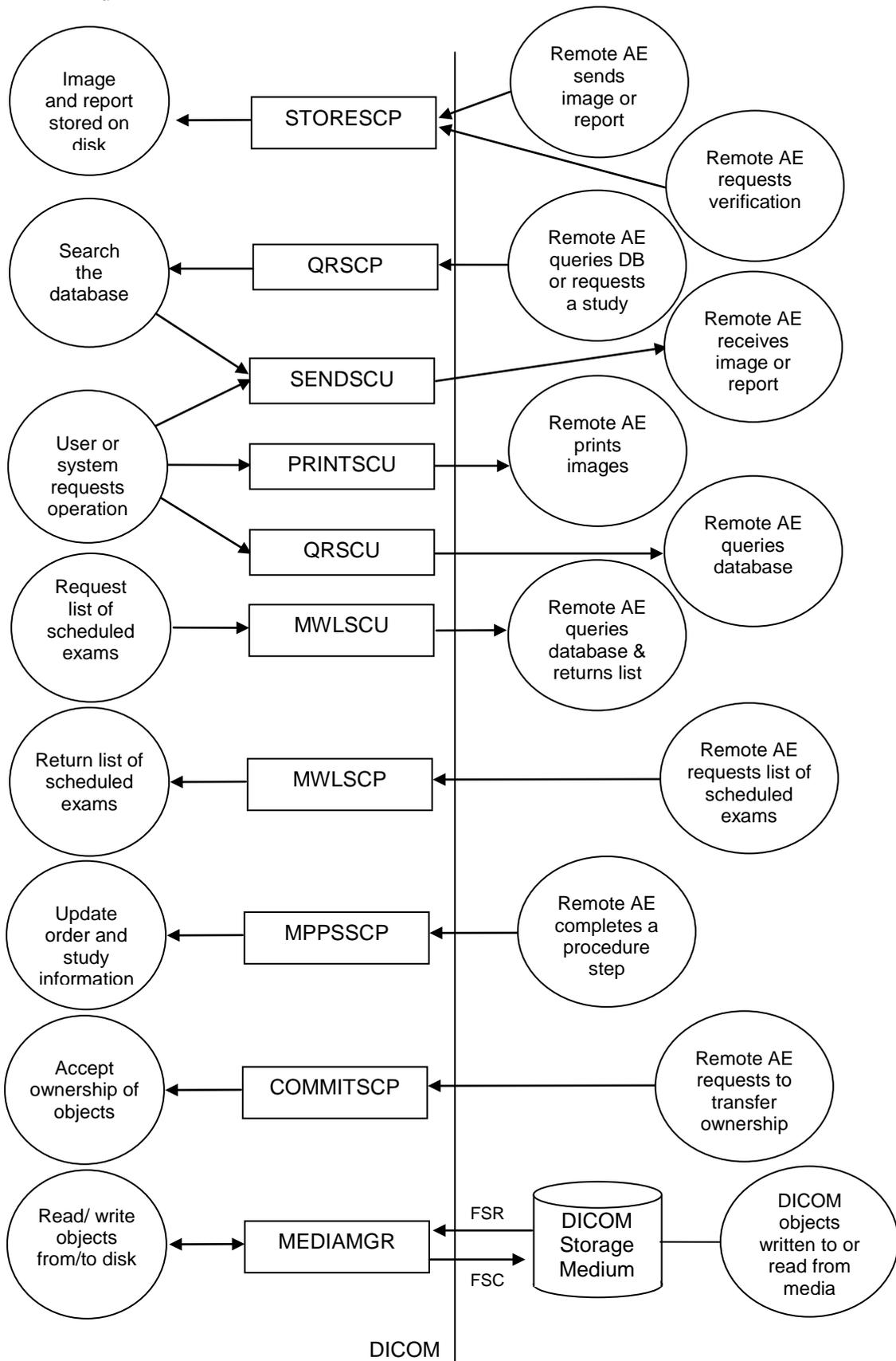
Figure 1.1-1 Application Data Flow Diagram
